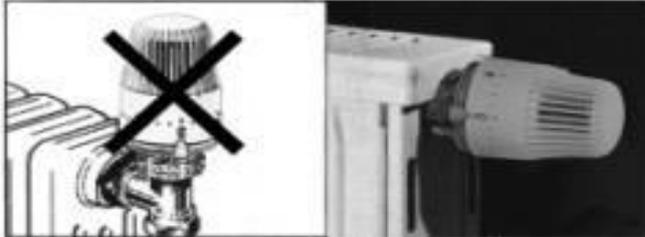
7. TRV's should not be obstructed by curtains or radiator covers and should not be positioned in direct sun light, preferably not installed vertically or in narrow corners as its sensor will read a high temperature and close the valve earlier than required.
